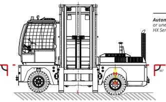
**Automatic deck-levelling:** Even on difficult or uneven ground conditions, Baumann HX Series sideloaders keep loads level.
